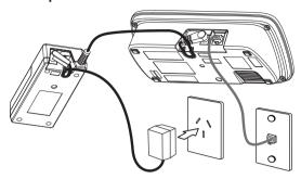
The BP-100 battery box is connected in-line between the base and AC adaptor of a compatible telephone.
