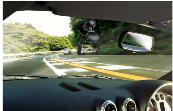
With the help of advanced accident recording 'black box' technologies, a built-in G-sensor and Collision Detection Mode, the camera identifies any changes in motion to instantly trigger recording. In an accident, this lets drivers see how the collision happened and analyse the direction of impact.
